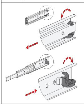
Telescopic slides can have an integrated self-retracting mechanism, which improves considerably the ease of use when closing the extensions.
