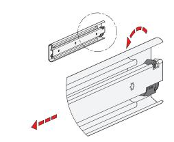
Telescopic slides GN 1432 have an integrated self-retracting mechanism, which improves considerably the ease of use when closing the extensions.
