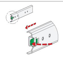
Unlike locking devices, a latch secures the slides in the stop positions in a frictionally engaged way. Telescopic slides with latches are used when the slides need to be protected against independent extension or retraction, for example, due to a tilted position.
