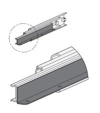
Support brackets on the inner slide are available on request for some slide variants, even in small quantities. The support bracket is used for simple fastening, for example, of a drawer, if side mounting is not possible. Fastening occurs by means of through-holes that are arranged at a right angle in the bracket.
