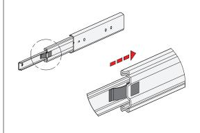
The locking function is noticeable by a slight resistance of the slides in the end positions, which has to be overcome on opening and closing. The locking device in the back stop position is usually integrated into the rubber stop function, making additional components unnecessary.
