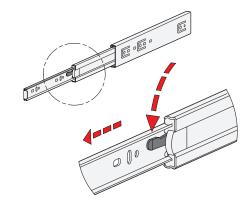
Type F has additionally a detach function through which the extension slides can be completely separated from one another in the area of the middle and inner slide. This feature not only facilitates mounting. It also allows the extension to be quickly removed, for example, when frequent maintenance work is performed on the components located behind.
