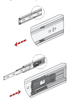
Telescopic slides GN 1414 have a dampened self-retracting mechanism, which is also called "soft-close". The dampened self-retracting mechanism is divided into two main functions and offers the best possible ease of use on closing the extension.
