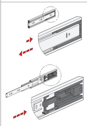
Telescopic slides can be fitted with a "push to open" or "touch to open" mechanism. In addition to ease of opening, the system allows you to have drawers without a front handle. This makes it easy to achieve a sleek, high-end appearance.
