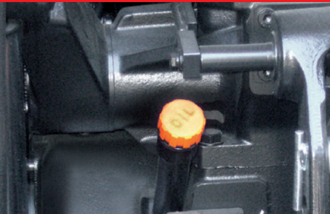
Application of SFP+a filler breather cap with splash guard and dipstick.
