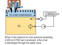
When in the reservoir a depression around 0.030 bar is produced, a flux of air entering the reservoir through the suction valve takes place.
